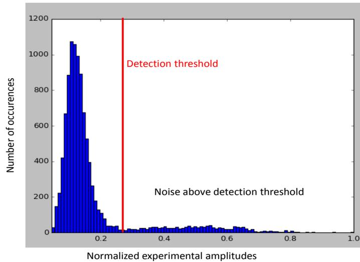
**Fig. 8.** Computation of PFA: histogram of backscattered noise.
