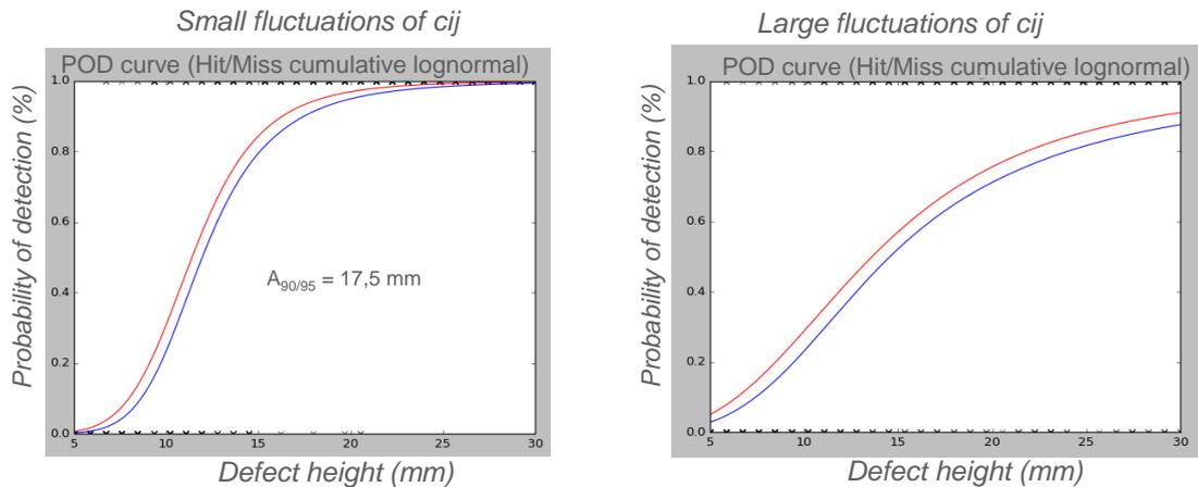
**Fig. 5.** Model-based POD curves computed in CIVA on notches normal to back wall, taking into account fluctuations of pipe thickness, when the stainless steel grade is known (i.e.  $c_{ij}$  vary feebly, left), or not (i.e.  $c_{ij}$  vary strongly, right).
