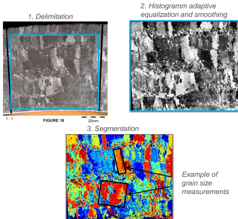
**Fig. 2.** Steps of image processing aimed at automatically computing the mean grain size in a given region of the component, using a macrograph.
