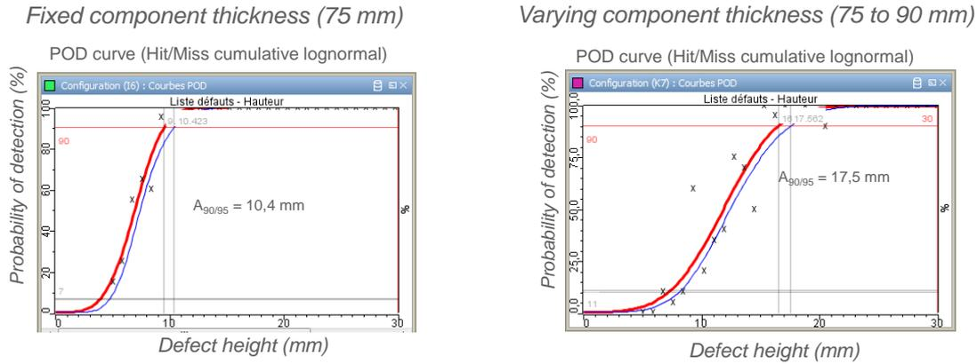
**Fig. 4.** Model-based POD curves computed in CIVA on notches normal to back wall when the component thickness is known and fixed (left), or when it varies from 75 to 90 mm (right). In both cases, delay laws are computed assuming the thickness is 75 mm.
