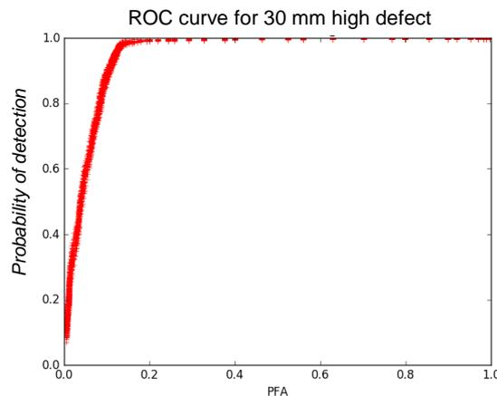
**Fig. 9.** ROC curve computed using experimental PFA and model-based POD curve (taking into account the fluctuations of incident wave due to grain size, and with small fluctuations of elastic constant and fixed wall thickness 75 mm).
