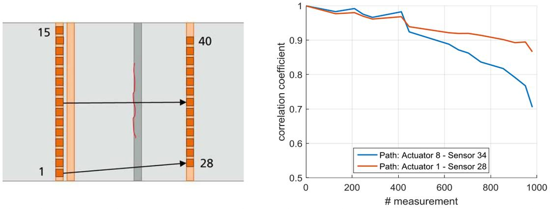
**Figure 4** Left: Draft of the numbering of the transducers within one of the reflection rings (1 to 15) and within the transmission ring (28 to 40) including the welded seam, a crack and two possible paths. Right: Correlation coefficient over 980 measurement for the given paths. The coefficient is determined by comparing the baseline and the current measurement.
