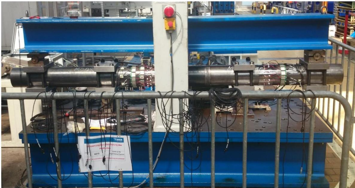
*Figure 2 Test stand of the 4-point bending tests at IMA Dresden.*
