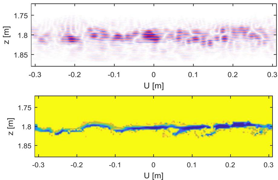
**Figure 5** Top: Results of the imaging method based on Fresnelvolume-Migration for one test crack. Bottom: High contrast photography of the corresponding crack to visualize the shape of the crack.
