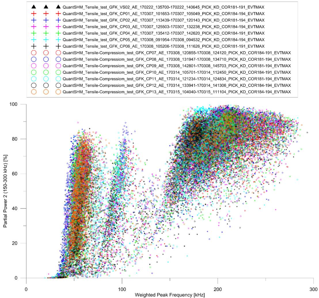
*Figure 7 Results of the AE measurements of the tensile tests with the GFRP samples as described in section 2.1. The clustering in the weighted peak frequency vs. partial power space of the acoustic events is based on the work by Hönig et al. in [7] and by Sause in [8].*
