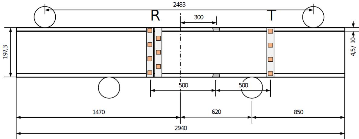
*Figure 1 Dimensions of the steel pipelines used for the 4-point bending tests in section 1.1. All dimensions in mm.*
