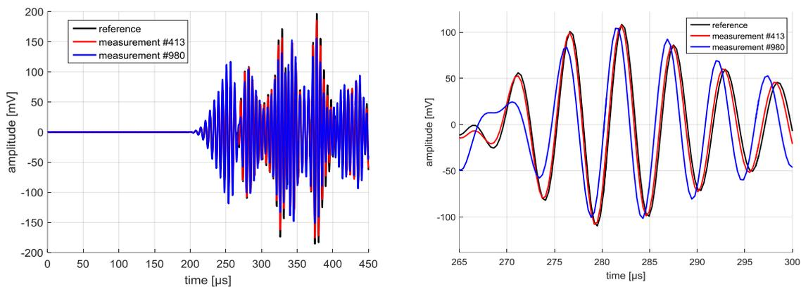
**Figure 3** Time signals of the pitch-catch measurements in section 1.1 on path actuator 8 to sensor 34, cf. **Figure 4**. Left: The whole signal after a recorded time of 450  $\mu\text{s}$ . Right: Zoom into the time interval from 265  $\mu\text{s}$  to 300  $\mu\text{s}$  which corresponds to the  $L(0,1)$  wave mode.
