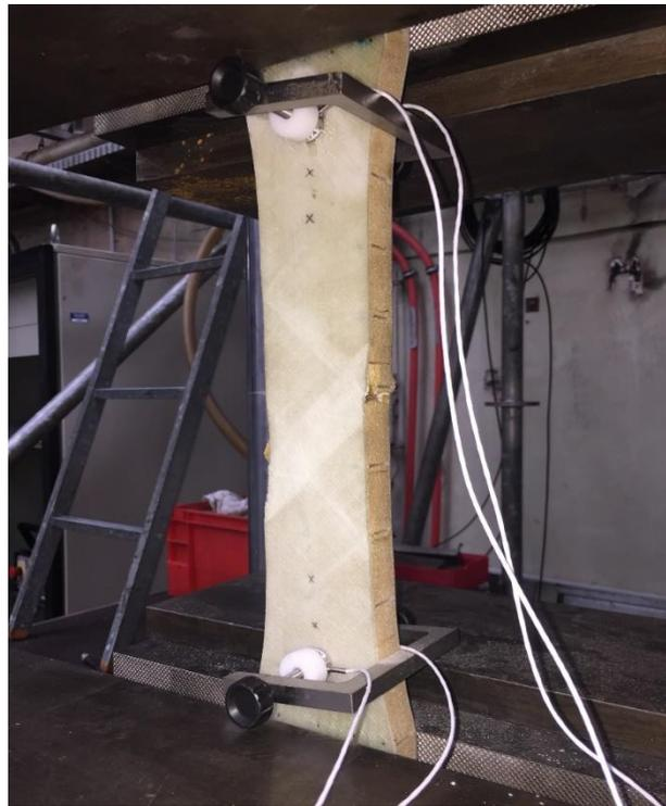
*Figure 6 Test stand of the tensile test at IMA Dresden.*
