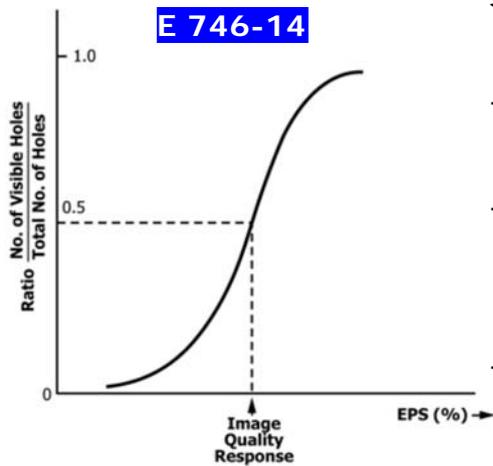
FIG. 4 Graph Method for Determining RIQI
